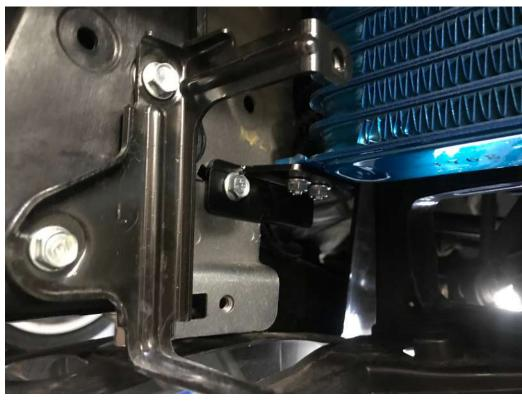
2.3a (update) Install the Oil Cooler brace on one side of the oil cooler core as shown in the picture below using provided M6 x 15mm P1.0 bolts and nuts
