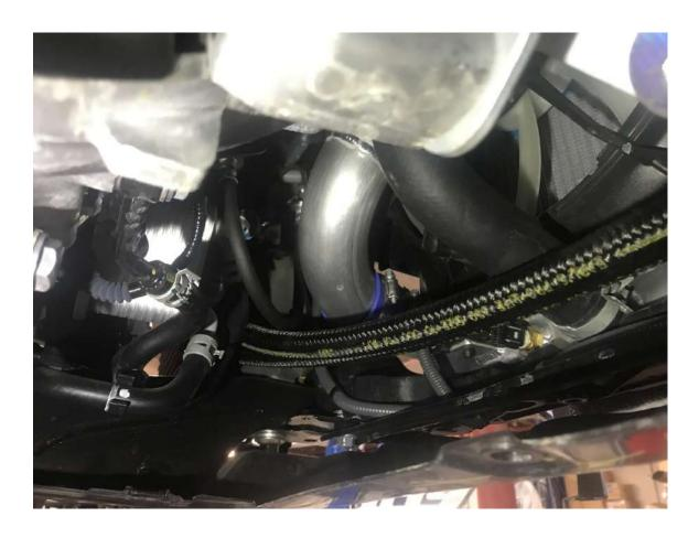
2.5 Secure the line to the radiator fan shroud frame behind the radiator as shown using zip-ties. Make sure to slide the thermo cover on the hoses near the downpipe. (not shown in the picture) (Parts used #11)
