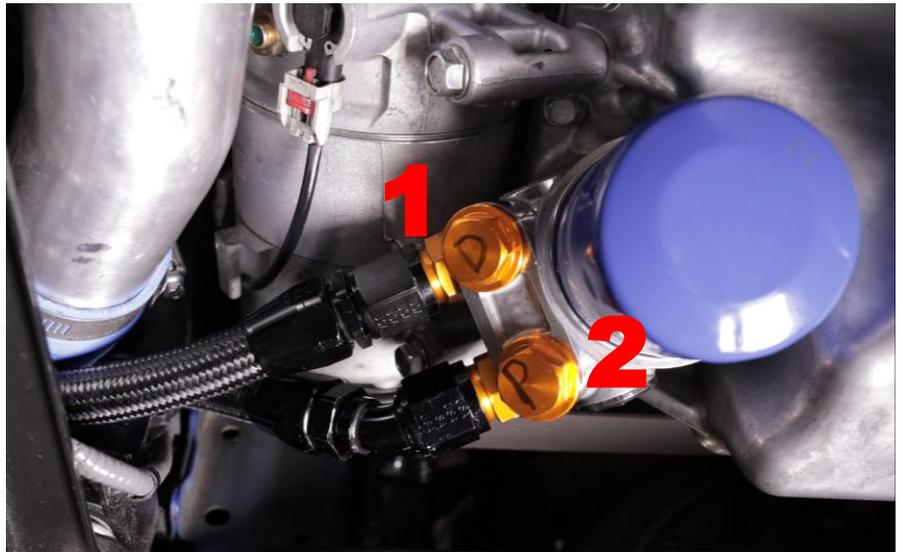
2.16 Once both fittings are threaded on hand tight use a 27mm socket and fully tighten the sandwich adapter block to the engine block. Recommended torque is 16 ft-lbs. At this time you can now install a new filter and fully tighten both -10AN hose ends.
