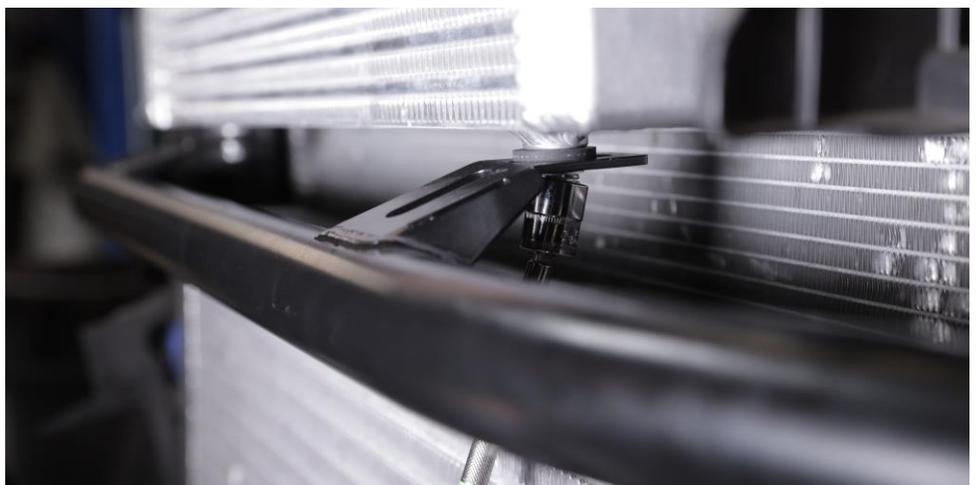
2.10 Install the 24" section of split corrugated plastic sleeve onto the longer hose to protect the hose from contact between the cooler core and condenser. Secure with the supplied zip ties. Using the longer oil hose, push the end with the straight fitting through the hole you cut in step 2.6 and route it as shown in the pictures below for the easiest fitment. (ITEM #4,12,13)
