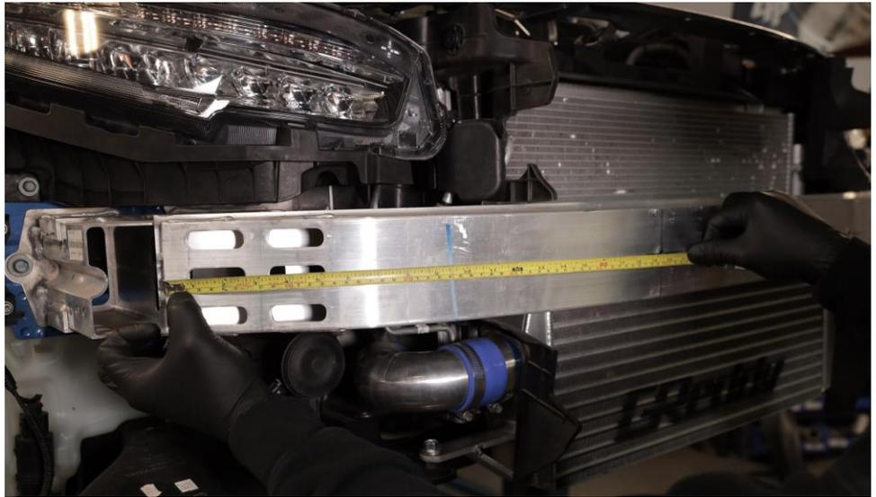
2.5 Drill the two marks that you made with at least a 5/16" drill bit. Make sure you hold the drill level top to bottom and centered left to right when going through the support beam. You may have to step up to a larger size drill bit if you cannot pass the bolt all the way through the support beam.
