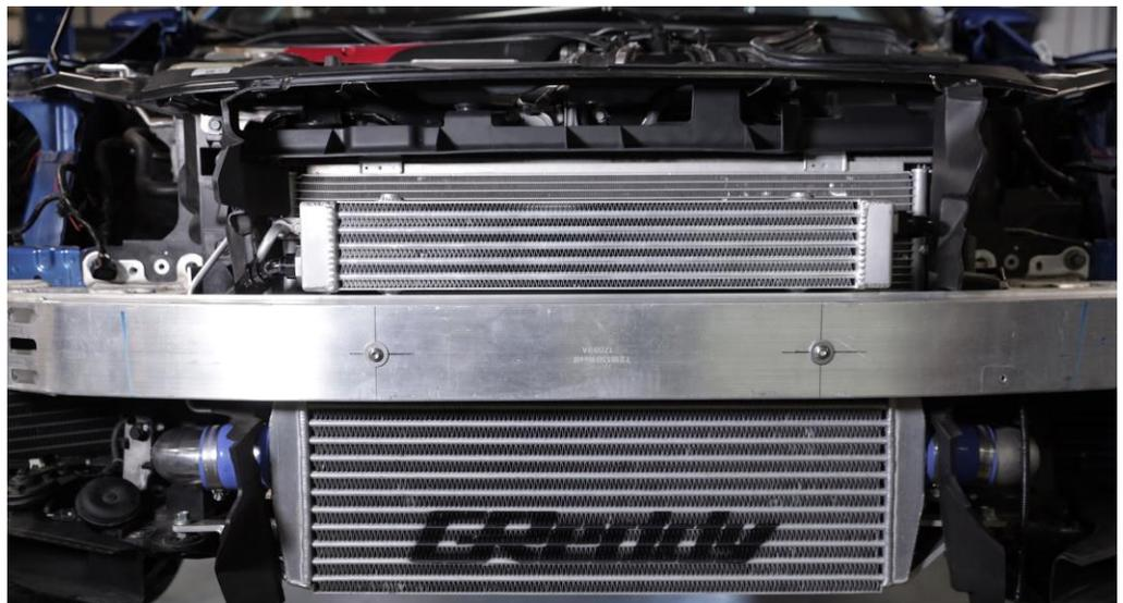
2.9 Mount the core to the GPP Front bumper bar with the lower oil cooler core port on the passenger side and the higher core port on the driver side. Place a M8 rubber isolator atop each tab of the bumper bar. Use the M8 bolts provided with the Koyo cooler core through the vibration washer, and thread into the bung on the bottom of the core. (ITEMS #1,10,11)
