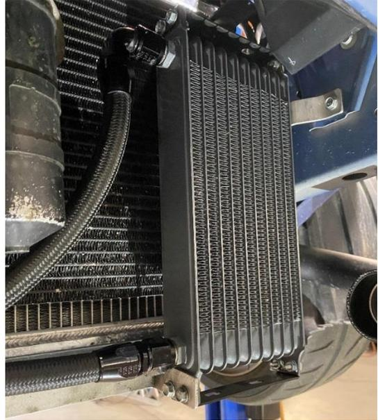
20. Attach hoses from engine block adapter to oil filter relocation adapter (ITEM #10, 11).
