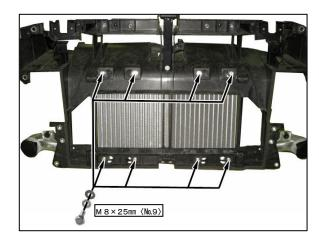
(3) Install intercooler air intake duct to the radiator air guide.
