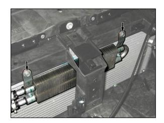
(9) Remove the window washer tank mount bolt.
