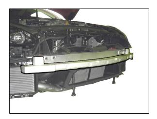
(4) Remove the bumper reinforcement.
