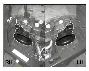
(3) Remove the impact foam from bumper reinforcement.
