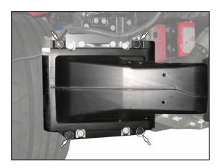
(2) Remove the air ducts from both sides.
