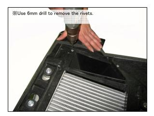
(2) Remove the intercooler from radiator air guide.
