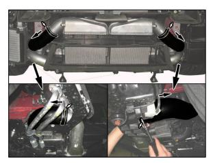
(11) Remove the radiator air guide, the intercooler and air intake duct.
