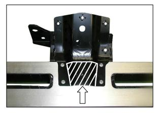
(2) Trim the Air Ducts approximately 5mm to keep from interfering with the intercooler.
