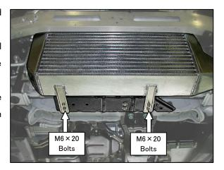
Wing the OEM bolts, install the new intercooler brackets in between the bumper reinforcement & OEM intercooler bracket as shown in the picture & diagram below.
