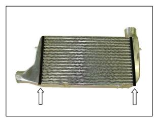
(3) Install the brackets as show below using the M8  $\times$  15mm bolts & washers.
