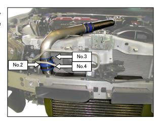
(2) Attach the Intercooler Outlet side to the OEM piping using part #'s 2, 3, & 4 as shown in the picture to the right.
