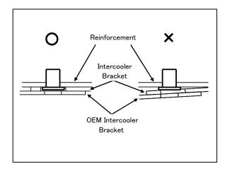
(5) Once you have adjusted the position of the new intercooler, tighten the bolts securely.
