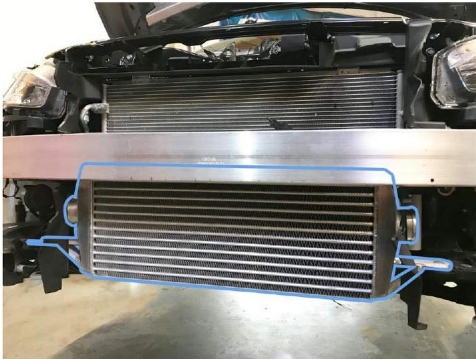
2.3 Insert the provided M10x40mm bolt(s) through the lower under frame through both sides of the factory intercooler rubber bushings and new Intercooler brackets. *\*(Some early kits will have a pre-welded stud that fits into the factory rubber bushing from above, instead of the provided #10. bolt.)*
