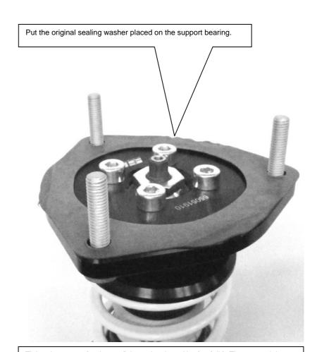
Tightening torque for the top fixing points is 25 Nm (18 ft-lb). The strut unit has to be installed according to manufacturers recommended settings regarding tightening torque and fixing specifications.
