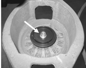
Mount the rear axle adjustment between spring and chassis. Remove the original spring supporting disc. You have to remove the rear axle adjustment to correct (screw up the threaded ring) the car height.
